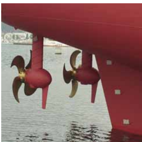
Photo: A fishing boat using an electric propulsion system (The stern bottom is slimmer with the absence of propeller shafts and rudders.)
