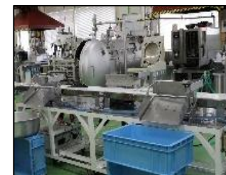
Automatic sorting using image sensing technology
