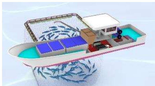
Illustration of a fish feeding vessel powered by a hydrogen battery
