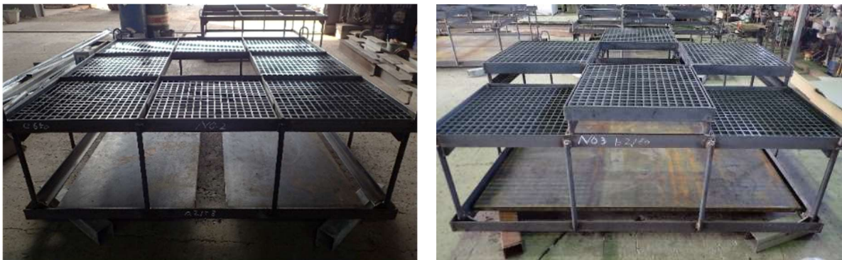
Figure 4: Shapes of two types (left: flat type, right: convex-concave type)
